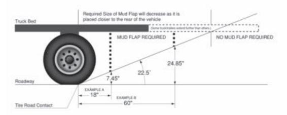
The above diagram can be used as a guide in determining whether your vehicle is required to have mud guards or flaps. Compliance may be determined by whether the rear wheels of a commercial vehicle throw road surface substances back and up at an angle greater than 22.5 degrees.
