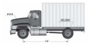
This vehicle has a bridge of 14'. Using the B/F chart, check the distance of 14' for two axles, finding a gross weight of 40,000 lbs. If this vehicle exceeds the formula weight of 40,000 lbs., the vehicle does not qualify for the bridge formula so only designated weights would apply.
