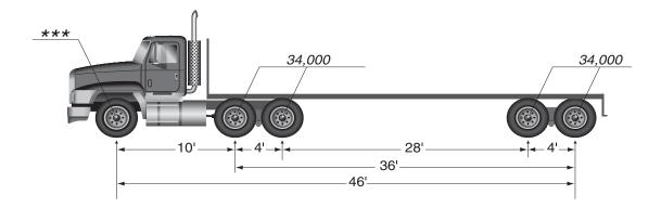
This 5 axle tandem tandem has an outer bridge of 46' (distance between axles 1 and 5). Using the B/F, this tandem tandem would be allowed a gross weight of 76,500 lbs. If this combination exceeds the gross weight of 76,500 lbs., it would be in violation. Also, the inner bridge on this vehicle is 36' (distance between axles 2 and 5). Using the B/F, this group of axles would be allowed a group weight of 66,000 lbs. If this group exceeds the weight of 66,000 lbs., the group would be in violation.
