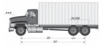
This vehicle has a bridge of 24' between axles 1 and 3. Using the B/F chart, this vehicle would be allowed a gross weight of 54,000 lbs. If this vehicle exceeds the B/F gross weight of 54,000 lbs., the vehicle does not qualify for the bridge formula so only designated weights would apply.
