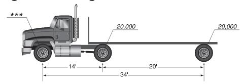
This combination has a bridge of 34' between axles 1 and 3. Using the B/F chart, this combination would be allowed a gross weight of 60,000 lbs. If this combination exceeds the B/F gross of 60,000 lbs., the combination would not qualify for bridge formula weights so only designated weights would apply (up to 18,000 lbs. on a single axle with proper tire size).
